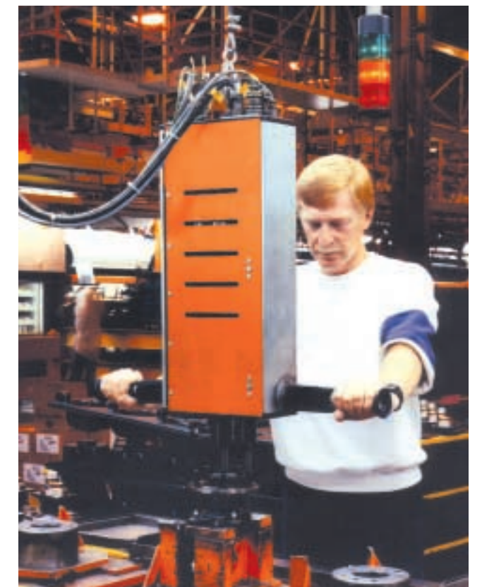
Repair bay operator is using a two spindle fixtured tool to fasten components of a wheel hub assembly.
