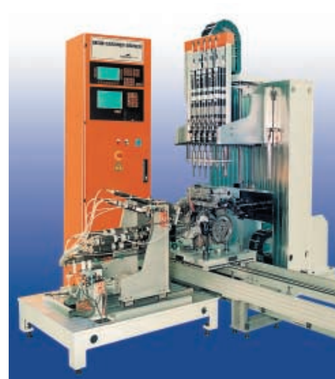
This GardoTrans installation shows a vertical system for floor level transport on the DaimlerChrysler Stuttgart 4 cylinder engine assembly line.
