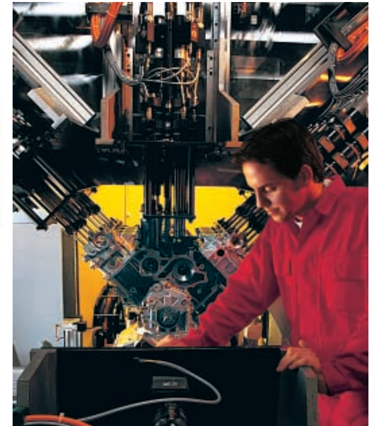
An automatic station on an engine assembly line uses two opposing electric power heads, each having 8 spindles, and a center power head of 6 spindles.
